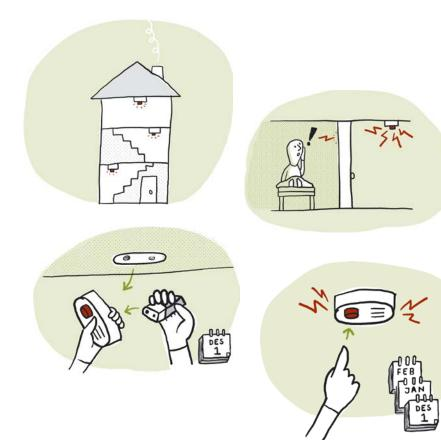
Every home must have at least one smoke detector on each floor. The smoke detectors provide an early warning in the event of a fire. You must be able to hear the alarm from inside bedrooms with the doors closed. The batteries must normally be replaced once a year. Test your smoke alarms regularly by pressing the test button.
